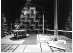
stricter (i.e., CE marking system, EMC Directives, and the JIS version of the EMC Directives), forcing us to install our own facility. We have also long needed a large, semi-anechoic chamber that has a low background noise.
